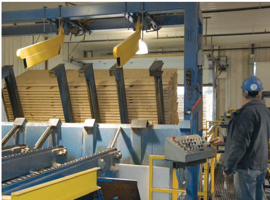
The Pleasant River Lumber mill has had a number of upgrades over the years, including a new planer infeed and a Tronco tilt hoist shown here. The infeed operator is Galen Elderkin.
